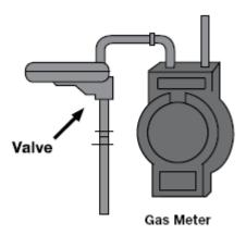
• To turn gas off, give the valve a quarter turn in either direction. When the lever crosses the direction of the pipe (see below) the gas is off.
